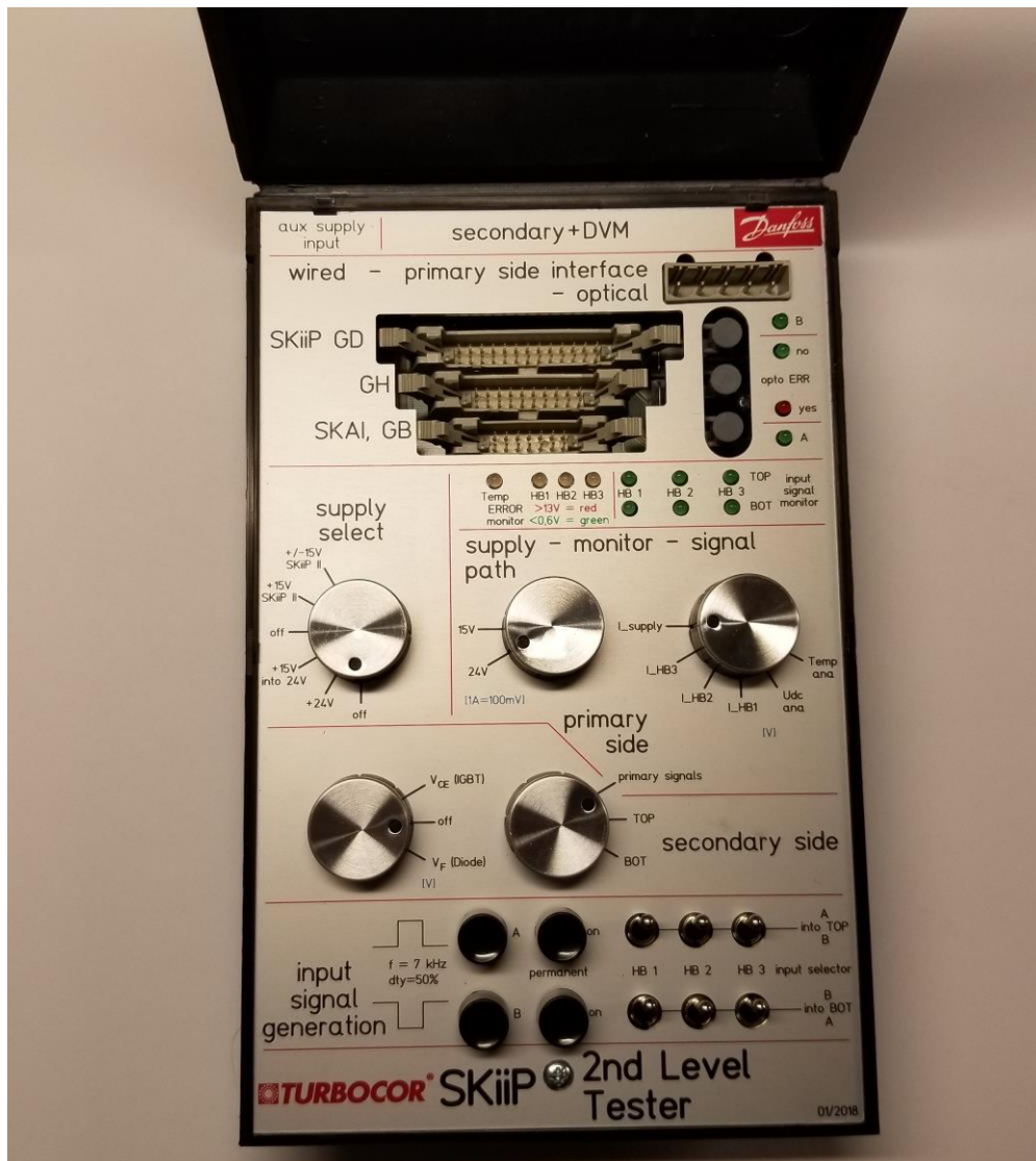
Figure 1 – New Compact Inverter Tester
