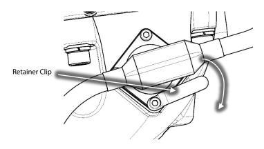
Figure 18 - Retainer Clip Rotation
