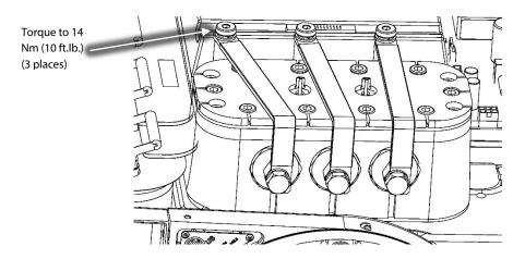
Figure 28 - Copper Tube Installation
