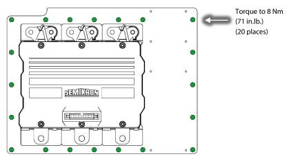
Figure 26 - Inverter Screw Locations
