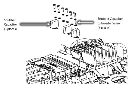
Figure 11 – Snubber Capacitor Removal
