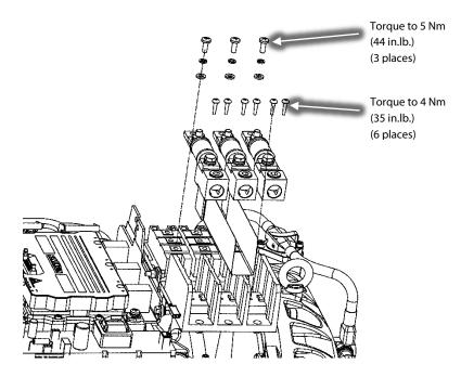
Figure 30 - Fuse Assembly Installation
