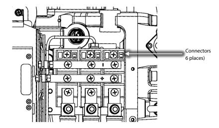
Figure 6 – Soft Start SCR Gate Cable Harness Removal
