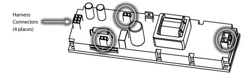
Figure 17 - DC-DC Harness Removal
