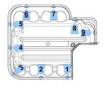
Figure 32 – Top Cover Torque Sequence
