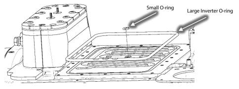
Figure 24 - Inverter O-ring Installation
