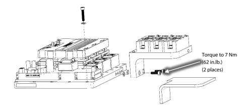
Figure 23 – SCR Cooling Manifold Installation
