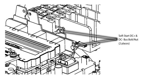
Figure 10 – DC+ and DC- Soft Start Harness Removal
