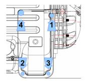
Figure 33 – Mains Input Cover Torque Sequence
