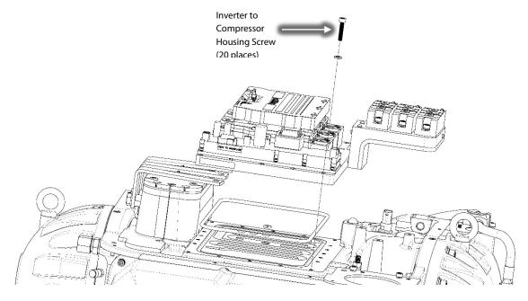
Figure 20 - Inverter Removal
