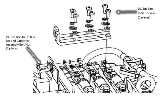
Figure 7 – DC Bus Bar Removal
