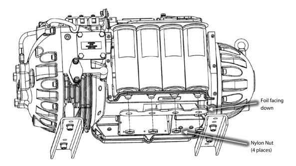
Figure 12 – Capacitor Nut Removal
