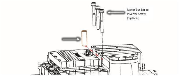
Figure 15 - Copper Tube Removal
