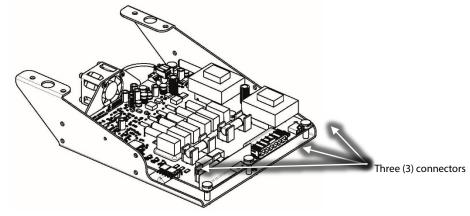
Figure 5 – Soft Start Harness Removal
