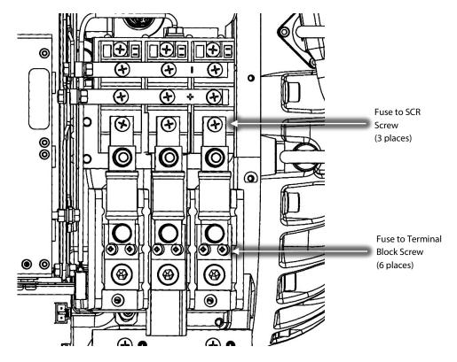
Figure 8 – Fuse Block Assemblies
