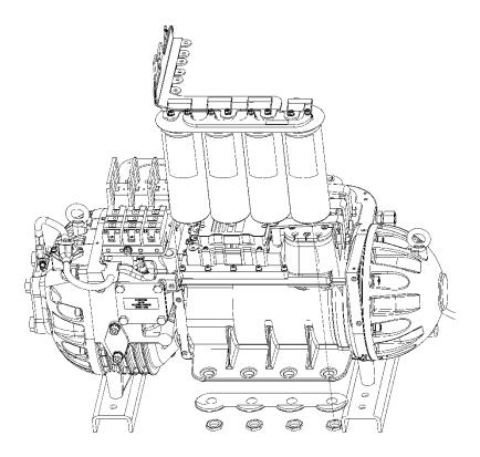
Figure 13 – Capacitor Assembly Removal
