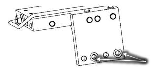
Figure 22 –SCR Cooling Manifold O-ring Installation
