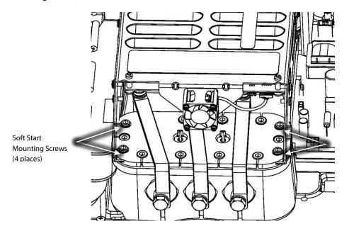
Figure 3 – Soft Start Mounting Screws
