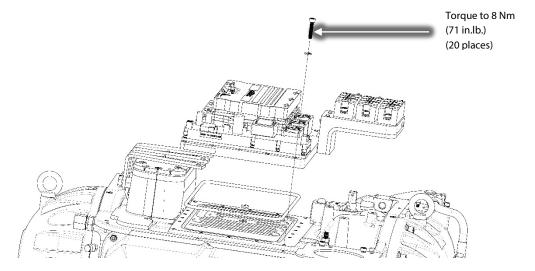
Figure 25 - Inverter Installation
