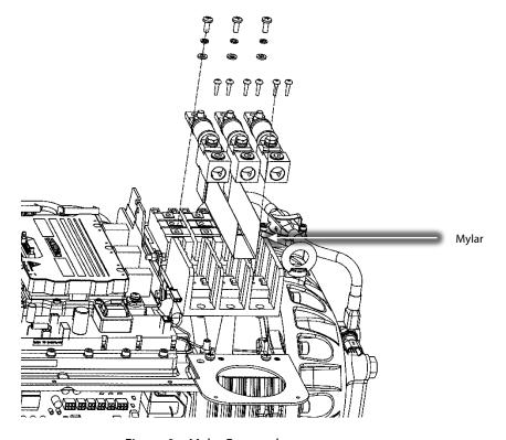
Figure 9 – Mylar Removal
