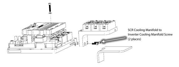
Figure 21 - SCR Cooling Manifold Removal
