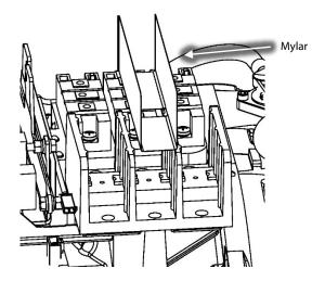
Figure 29 - Main Power Mylar Insertion
