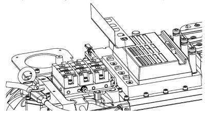
Figure 14 - Mylar Removal
