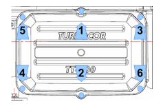
4. Follow the sequence twice. The first time, only fasten the screws to half way down to allow for adjustment. Torque to 13 in.lb. on the second pass.
