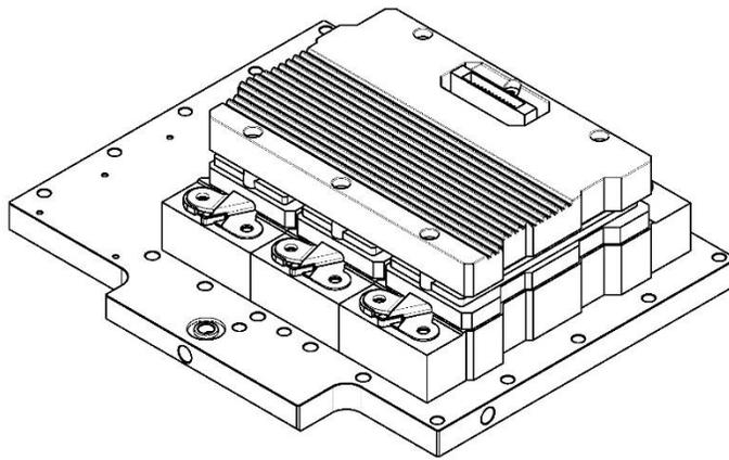
**Figure 1 – New 613-Type Inverter**
