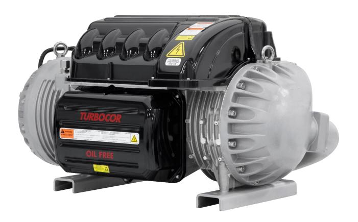
Two (2) models are available: TTH375 with a nominal capacity of 107 tons / 376 kW and TGH285 with a nominal capacity of 82 tons / 288 kW at typical air-cooled conditions. The TTH and TGH compressors provide a high-efficiency solution that enables an oil-free air-cooled chiller solution that can be deployed as a global platform.
