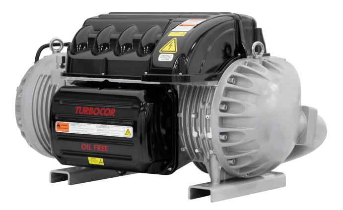
Two (2) models are available: TTH375 with a nominal capacity of 107 tons / 376 kW and TGH285 with a nominal capacity of 82 tons / 288 kW at typical air-cooled conditions. The TTH and TGH compressors provide a high-efficiency solution that enables an oil-free air-cooled chiller solution that can be deployed as a global platform. The TTH375 is available for use with R134a or R513A. TGH285 is available for use with R1234ze.
