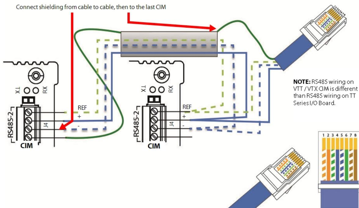
**Table 3-2 RS485 Data Cable Pinout for CIM**
