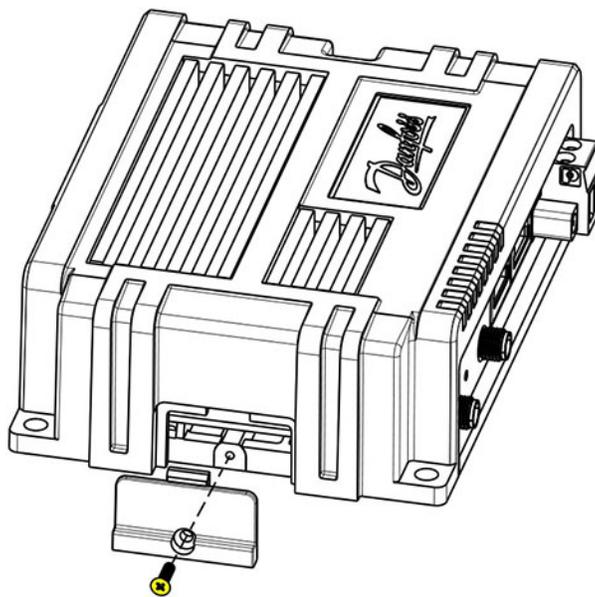
2. Insert the SIM Card into Slot 1 socket with the chamfered corner as shown in Figure 2-2 SIM Card Insertion.
