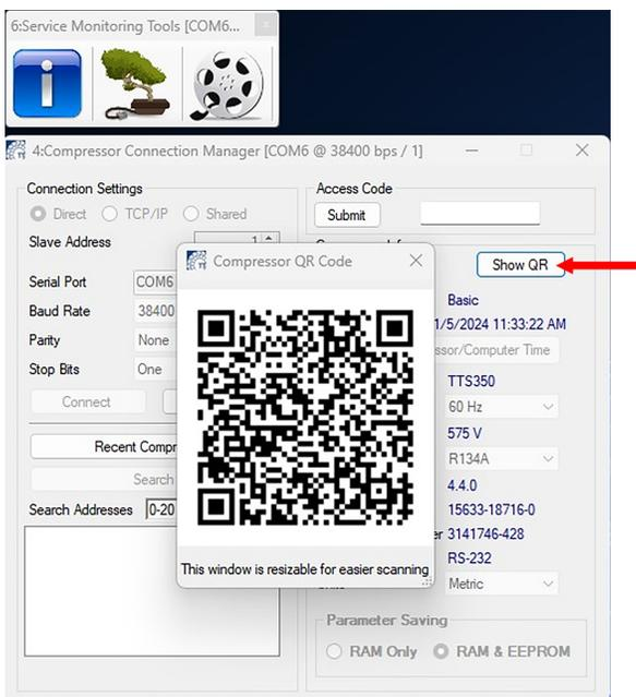
35. Position your mobile device over the QR Code located in the SMT until it appears in the scan window. Refer to Figure 4-28 Scan SMT Serial Number.
