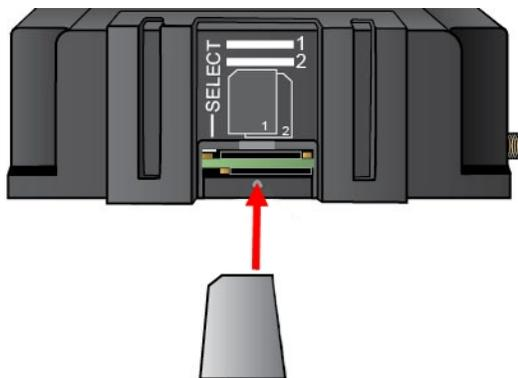
3. Reinstall the SIM Cover. Torque the fastener to no more than 225 mN m (2 in.lb.).
