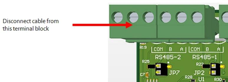
2. Utilize a RS485 to USB adapter cable (refer to Figure 6-2 SMT Cable Connection) to connect between the Compressor I/O Board or CIM to your computer. This connection will work the same as with RS232 connection. Refer to the [TT/TG Series Service Manual](#) for more information.
