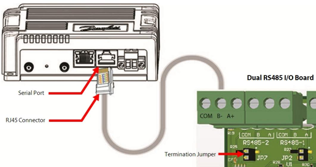
**Figure 3-2 Gateway to I/O Board Connection Pinout Reference (TT/TG Series Compressors)**
